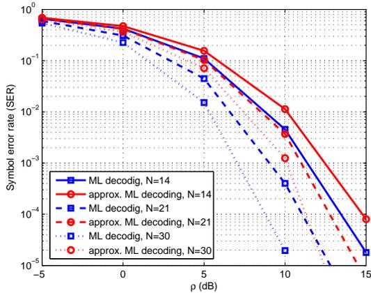
Fig. 3: Symbol error rate (SER) of the proposed coded diversity technique with ML and selected subset ML decoding schemes according to SNR in dB scale.  $M = 8$  and  $B = 1$ .
