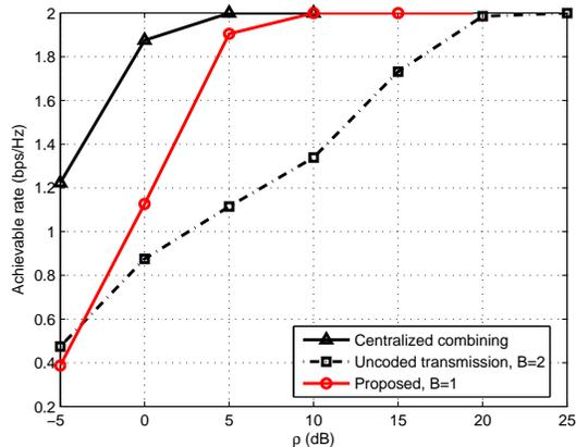
(b) Fading channel with normalized channel gain of  $|h_1| = |h_3| = 1.5$  and  $|h_2| = 0.3$ .Fig. 5: Achievable rate vs. SNR in dB scale with  $M = 4$ ,  $N = 3$ , and  $B = 1$ .
