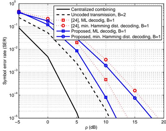
Fig. 2: Symbol error rate (SER) vs. SNR in dB scale with  $M = 4$  and  $N = 10$ . Each receive node of the proposed scheme and the scheme from [26] forwards  $B = 1$  bit per channel use to the fusion center while uncoded transmission relies on  $B = \log_2 M$  forwarded bits per channel use from each node.
