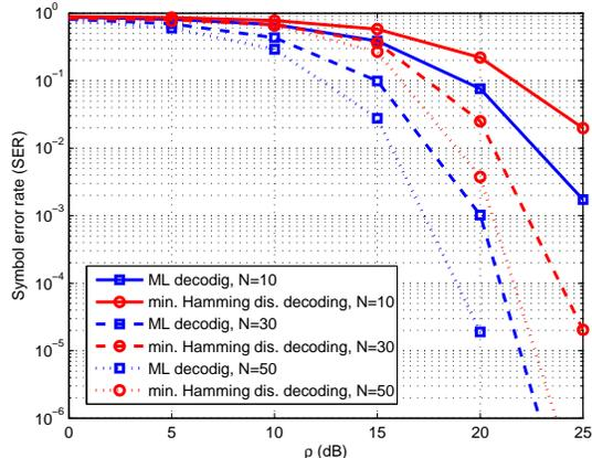
(b)  $M = 16$  (16QAM) constellation for  $S$  and  $B = 2$ .Fig. 4: Symbol error rate (SER) vs. SNR in dB scale with different values of  $M$ ,  $B$ , and  $N$ .
