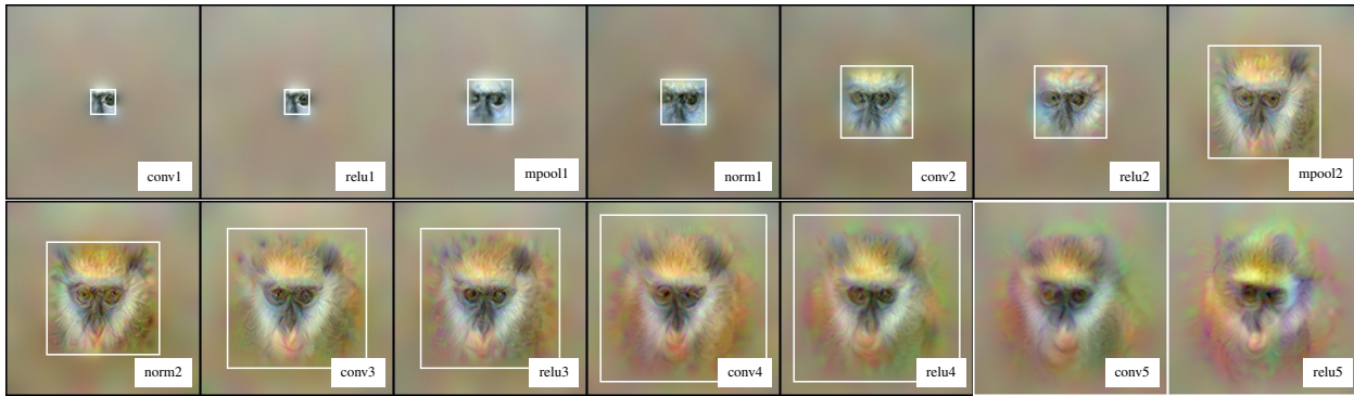
Figure 9. CNN receptive field. Reconstructions of the image of Fig. 5.a from the central 5 \times 5 neuron fields at different depths of CNN-A. The white box marks the field of view of the 5 \times 5 neuron field. The field of view is the entire image for conv5 and relu5.
