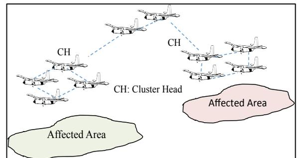
Fig. 4: Multi-Level Hierarchical Routing in UAV networks
