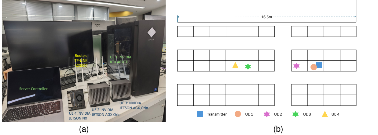
Fig. 9: (a) System components of WDMoE hardware testbed; (b) Geographical distribution of experiment devices.
