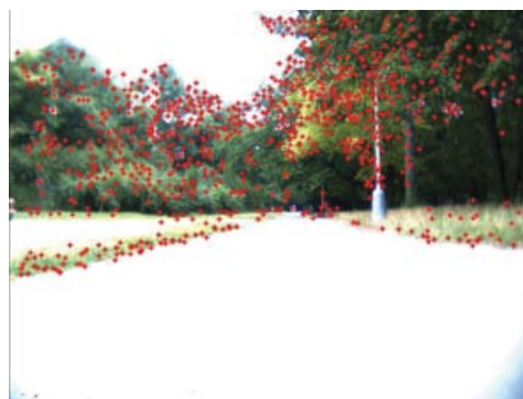
(b) Image captured by robot camera and detected SURF positions
