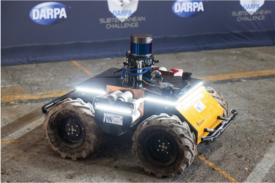
Fig. 4. The husky platform after leaving a muddy mine. Note the Robosense 3D lidar on the top and the gray carousel between the wheels. The carousel stores and releases the communication modules described in Subject. 4.5.
