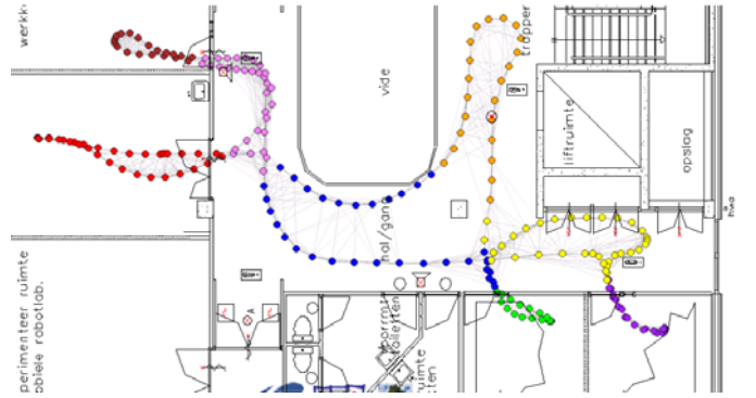
Fig. 5. The clustering found with the graph cut mechanism reflects the structure in the building
