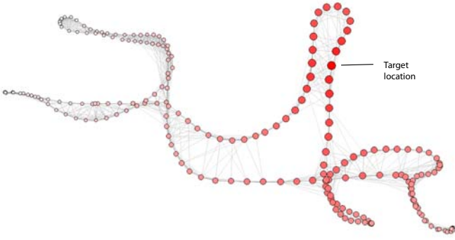
Fig. 6. A cost function is created on the basis of distances to the goal node
