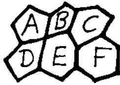
Figure 1. This set of cells has six adjacency sets of dimension 0: \{A\} , \{B\} , \{C\} , \{D\} , \{E\} , and \{F\} . The 1D adjacency sets are \{A, B\} , \{A, D\} , \{B, E\} , \{D, E\} , \{B, C\} , \{C, F\} , \{C, E\} , and \{E, F\} . The 2D adjacency sets are \{A, B, D, E\} , \{B, C, E\} , and \{C, E, F\} .
