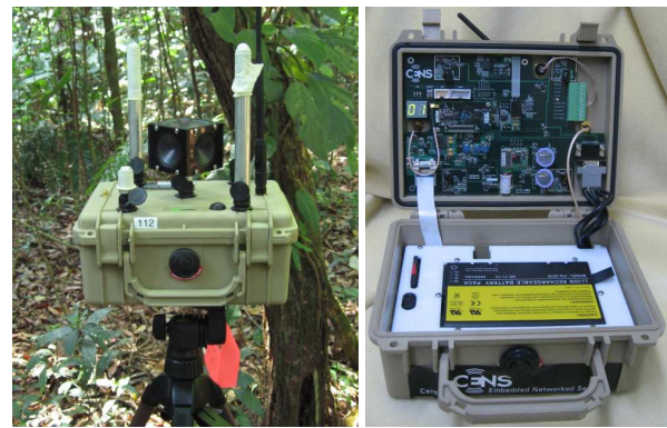
Figure 2: The Acoustic ENSBox Version 2, shown deployed near Chajul Station at left. A detailed description of both the hardware and software of this platform may be found in Collier (2010).
