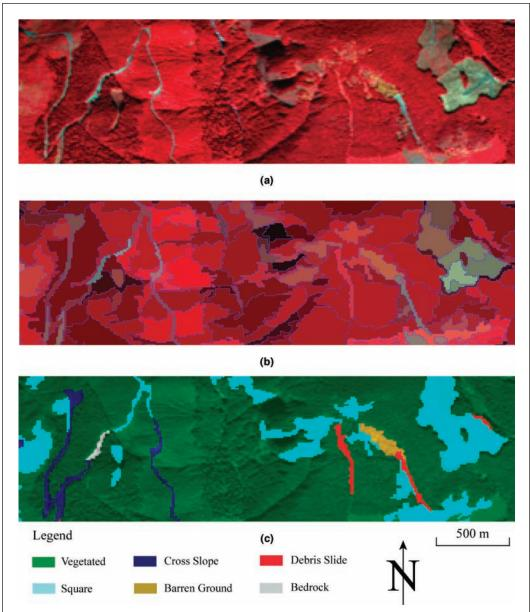
Plate 1. An example of the steps taken in the classification process. (a) denotes the raw imagery, (b) the imagery after segmentation into image objects, and (c) shows a portion of the classified imagery. Note the successful discrimination of the debris slides on the right of the image from the roads on the left. Part of the road system has been misclassified as bedrock.
