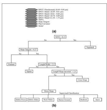
Figure 2. Classification schematic showing data layers (a) and the classification hierarchy (b). Note: not all image layers are used in the supervised classification, see text for details.
