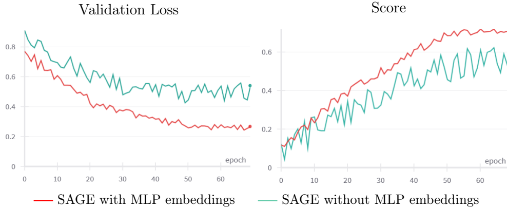
Figure 6.1: The plot illustrates the training curve of the comparison of using MLP-generated embeddings versus feeding the raw one-hot-encoded data to the SAGE backbone network.
