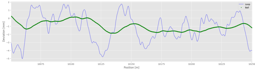
Figure 2.5: Overdamping \zeta = 5 . Blue curve: rail’s lateral irregularity. Green curve: ball’s movement trajectory.
