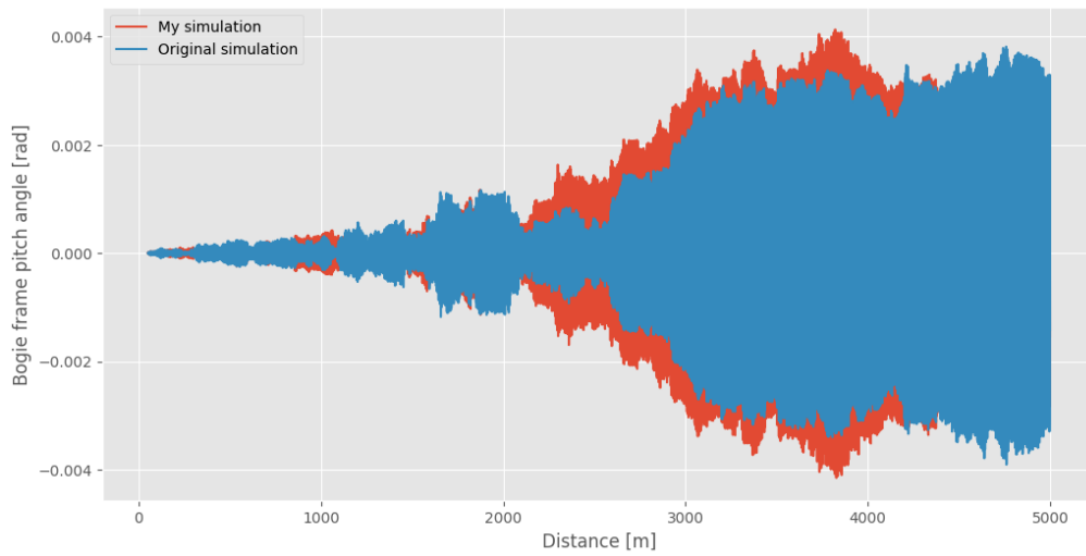
Figure D.13: The consistency of bogie frame's pitch angle.
