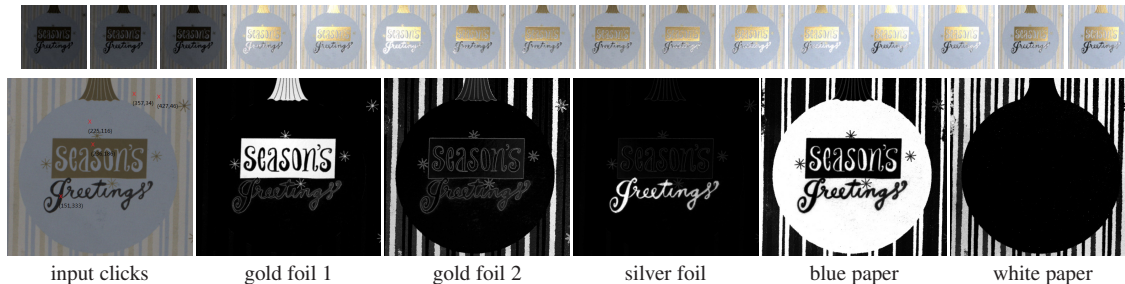
Figure 2. KNN matting on material matting using the sg dataset. Original images at top; bottom shows sparse user input (5 clicks; one per layer) and the five layers automatically extracted. Our result distinguishes the two different gold foil layers despite their subtle difference in materials (where they were combined in [10]). Figure best viewed in electronic version.
