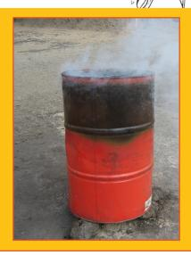
A 55-gallon oil drum can be used as a kiln to make charcoal. In order increase the airflow through the drum, cut several small holes in the bottom. In the other end, cut a large square opening for filling the kiln with cobs. You will also need a piece of sheet metal for a lid to cover the hole on the top. When starting the burn, the drum should be placed on top of three stones, so that air can flow in through the holes in the bottom.
