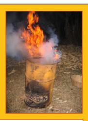
Light the drum at the bottom of the hole formed by removing the stick. After about ten minutes, ignite the smoke, to make the fire burn more cleanly.
