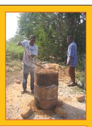
Cover the drum with the metal lid. Wait about two minutes then carefully remove the stones from under the drum. Seal the bottom edges and the top with sand. Wait at least two hours before opening the drum
