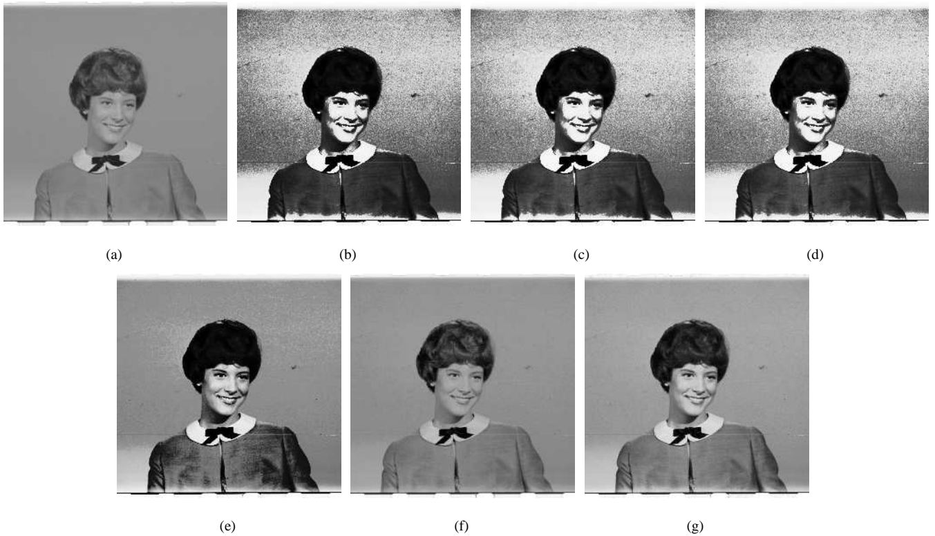
Fig. 6. Contrast enhancement results for image Girl : (a) original image; (b) GHE; (c) BPHEME; (d) FHSABP; (e) HMF; (f) CEBGA; and (g) proposed.
