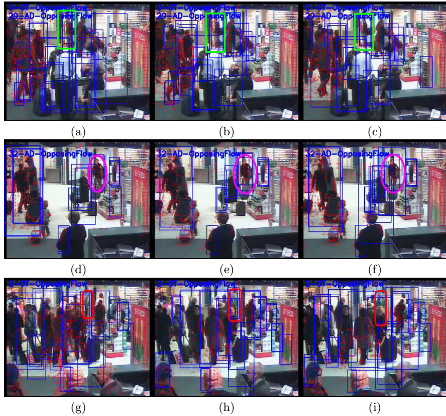
Fig. 5. Sample opposing flow event detection results. (a-c) True positive; (d-f) false positive; and (g-i) false negative. (For visibility, objects associated with true positives are marked with green rectangles, false positives are marked with magenta ellipses and false negatives are marked with red rounded rectangles).
