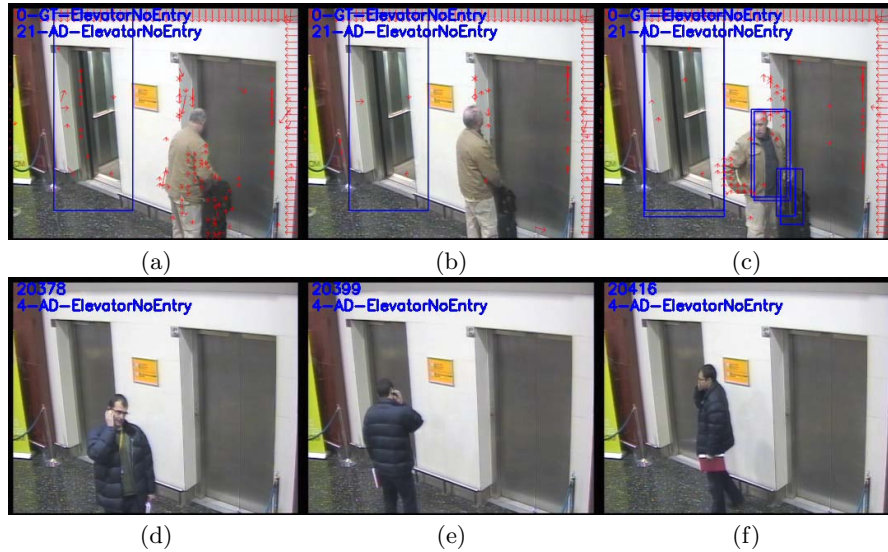
Fig. 4. Sample elevator no entry event detection results. (a-c) True positive; and (d-f) false positive.
