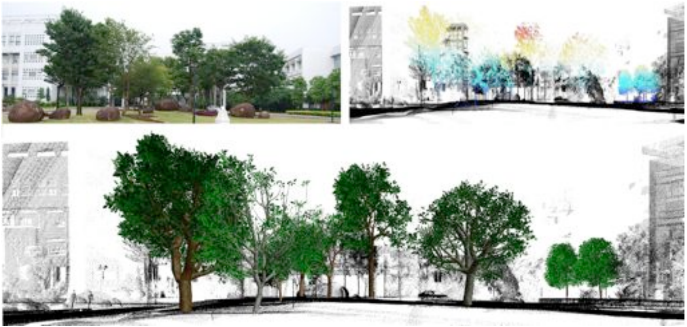
Figure 11: An urban scene with more than 10 million points, about 200,000 of which capture 20 trees. The trees are of various species, some with low-quality captures. The top two images show a photo and the point scans of the trees, colored by height. Note that the trees are not pre-segmented from the rest of the data. Our method automatically extracts the structures of the trees from the rest of the data (bottom) in about 30 minutes.
