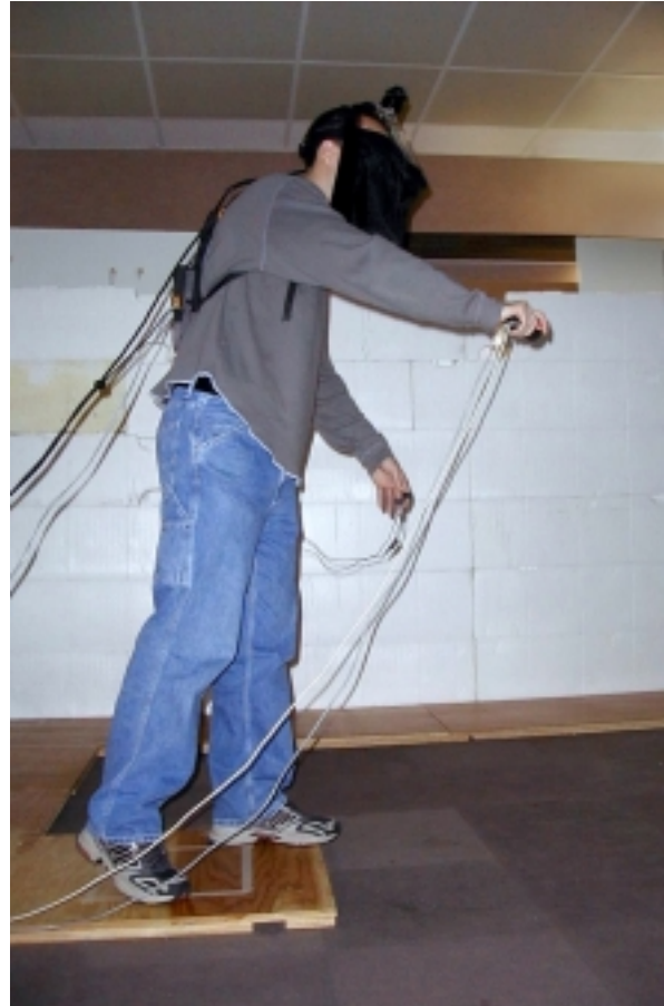
Figure 1.7. A subject drops a block into the virtual pit. He is standing on the edge of the 1.5-inch wooden ledge. The physiological monitoring equipment is attached to his left hand.
