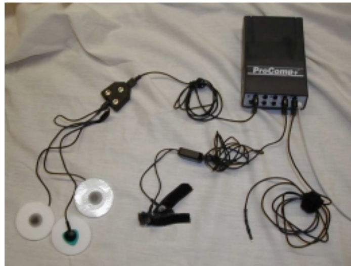
Figure 3.2. Procomp+ device. From left to right: the electrocardiograph, skin conductance, and skin temperature sensors.
