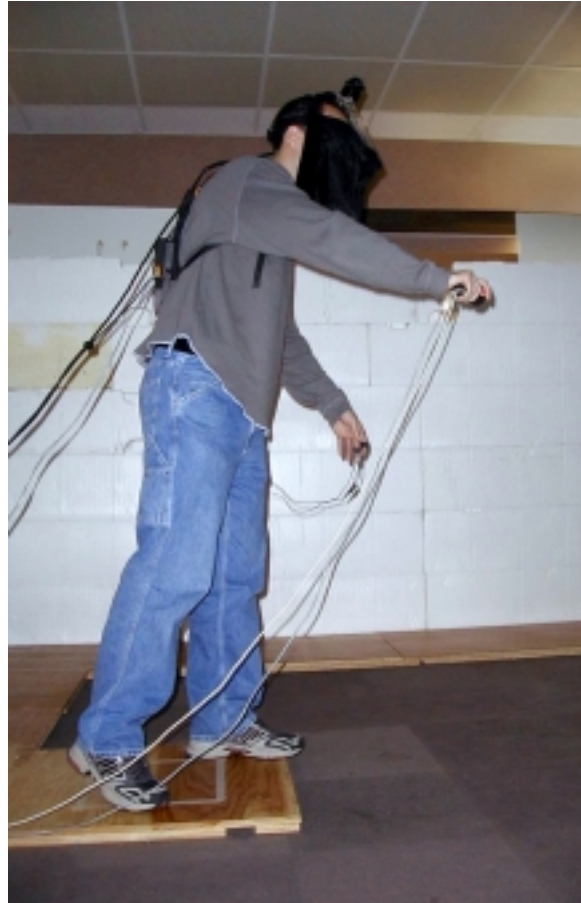
Figure 3.4. A subject drops a block into the virtual pit. He is standing on the edge of the 1.5-inch wooden ledge. The physiological sensors are attached to the left hand.
