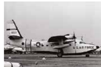
Above: SA-16A Albatross amphibious aircraft as used at RAF Bentwaters in 1951 to rescue aircrew stranded at sea. The Albatross could use runways as well as the open sea.
