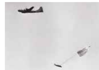
Above: Boeing SB-29 Superfortress demonstrating the dropping of the lifeboat by parachute. Having located the downed pilot, providing a life-saving boat to await rescue from a rescue ship was key to survival.
