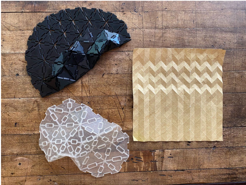
Figure 3. 3D printed and laser scored kinetic model samples
