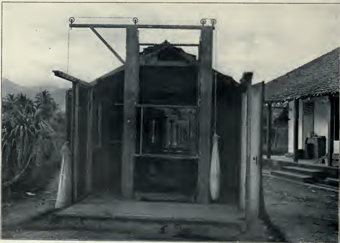
THE INTERIOR OF THE 60-FOOT CAMERA. Photographed by W. W. Dinwiddie.
