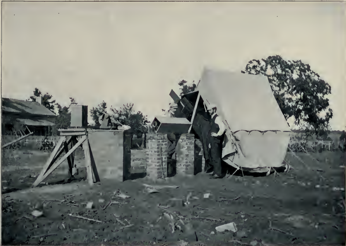
THE 10-FOOT CONCAVE GRATING SLIT SPECTROGRAPH AT GRIFFIN, GA. Photographed by W. W. Dinwiddie.
