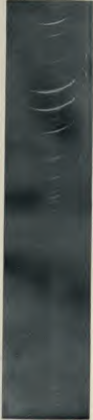
TOTAL SOLAR ECLIPSE OF MAY 17, 1901. THE ULTRA-VIOLET PORTION OF THE SPECTRUM AS PHOTOGRAPHED WITH THE SPECTROGRAPH AT FORT DE KOCK, SUMATRA. NEGATIVE 2, 5 SECONDS EXPOSURE. ORIGINAL SIZE.
