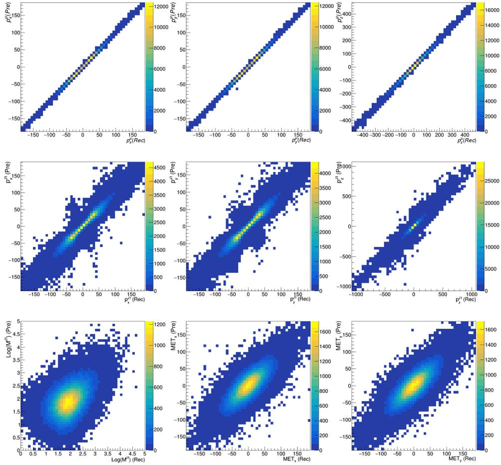
Figure 9: Distribution of input features predicted by the model as a function of the corresponding quantities from detector simulation.
