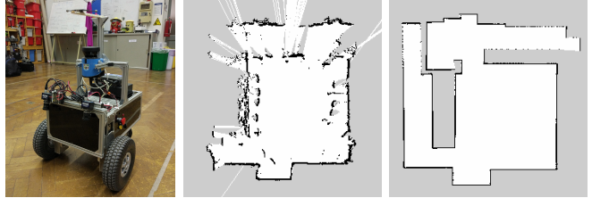
Fig. 8: The robot Robocom (left). The map built by Robocom in the AIRLab (center). The map built in a simulation run (right).
