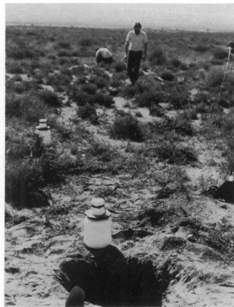
Fig. 1. View of the terrain typical to this study. In the foreground is a receiver in its protective case. The antenna is in the upper housing and a ground plane separates it from the electronics below. The data collection unit can be glimpsed beside the crouching figure in the background.
