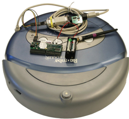
Figure 3: iRobot Roomba vacuum cleaner robot attached to a Gumstix computer.
