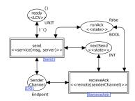
Fig. 2: The Sender principal module
