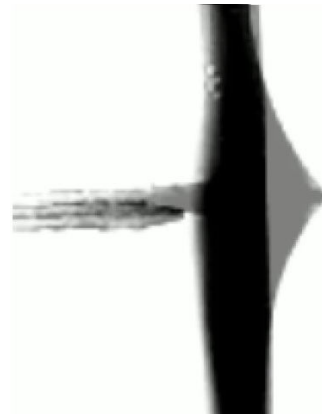
Figure 2: Overlay of a colored gelatin layer before penetration with a needle. The darker image shows the layer before needle contact. The lighter image shows the deformed layer.
