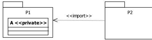
Fig. 2. Import of a private class through a single package import
