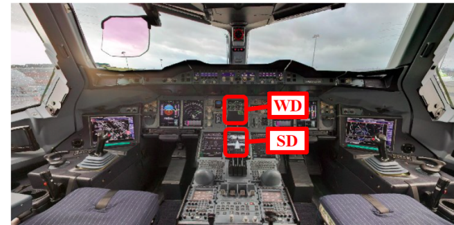
Figure 5: WD and SD in the cockpit of the A380
