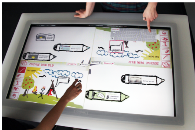
Fig. 4: Divided Screen – Personal Working Areas: The users are able to work on four areas on their own or collaboratively. This means that users work on their personal working area, but when cooperating with another visitor they draw in their respective drawing areas simultaneously.
