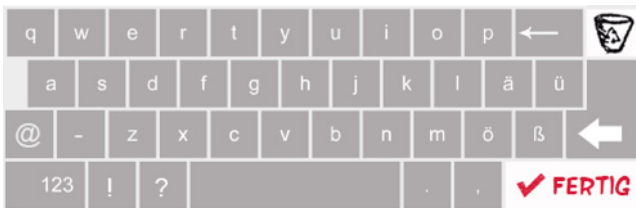
Fig. 9: The improved keyboard design as a result of the laboratory test.
