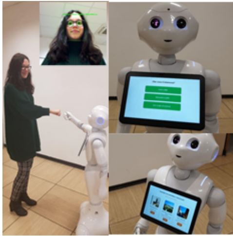
Figure 2: An example of interaction of a young woman with Pepper. In the upper part of the Figure the result of real time gender and age estimation is shown.
