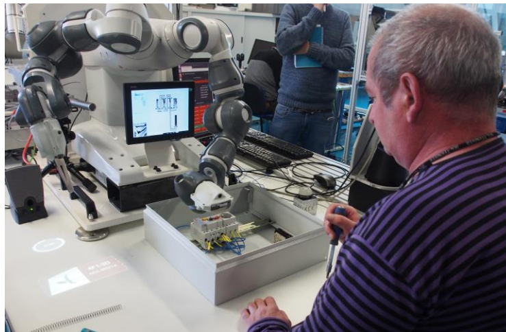
Figure 1: Worker with intellectual disabilities assembling an electrical cabinet in collaboration with a cobot. The robot checks the cables the worker has just connected and informs the worker if an error is found, giving them an opportunity to correct it.
