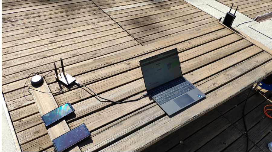
Figure 2: User devices used for the testing. Rokubun MEDEA navigation computer has been placed at the top left side of the table (test point T8). Smartphones such as Google Pixel 4 has been used as well. A Compulab WILD Access Point has been placed at the top right side of the table (test point T7)
