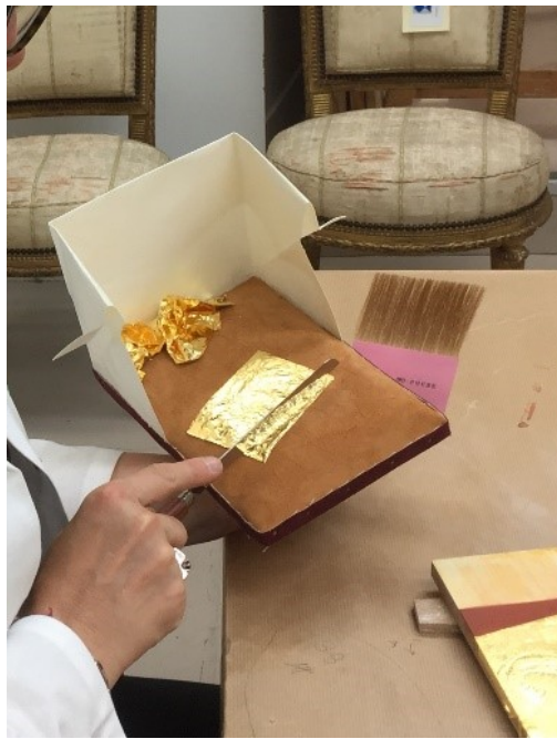
(a) Gold foil on a gilders cushion, cut with a trowel before being placed on the substrate using the gilder's tip (pink) ©C2RMF/Stéphanie Courtier
