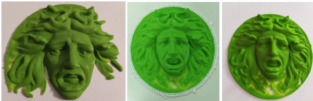
Figure 6: Left: Third model after printing without support material. Center: Third model with support material. Right: Third model after printing with support material.
