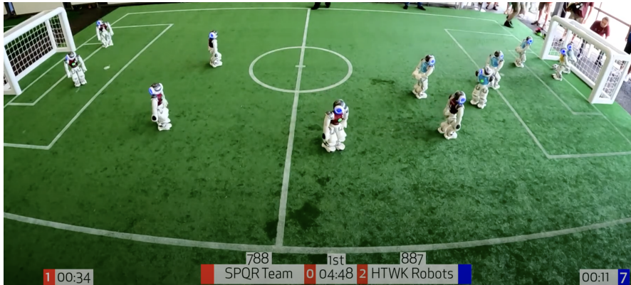
Figure 1: Frame from the quarter-finals of the RoboCup SPL 2023 between SPQR and HTWK teams. Above the names of the teams, the counters of the exchanged packets for each team are shown.
