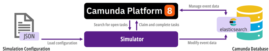
Figure 1: Interactions of the simulator components with each other.
