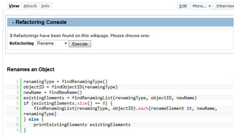
Fig. 5. A refactoring script in the wiki written in Groovy, which renames an object globally.
