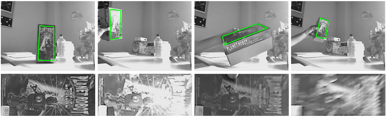
Fig. 9. registration of a planar template through illumination variations. First row: frame 0, 200, 400 and 600. The green rectangle represents the rectangle from the template image transformed using the estimated homography. Second row: projection of the templates for the same iterations in the reference image.
