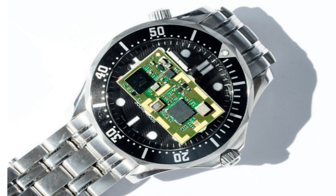
Multi-year GPS tracking with a watch for size comparison. A student manually did the amazing soldering work (metric SMD 0.4 mm x 0.2 mm).
