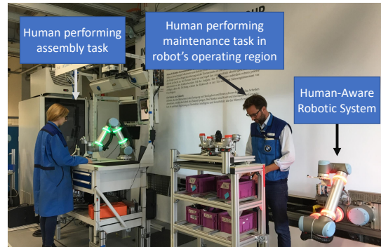
Fig. 1: The human-aware robotic system delivering parts to a human associate during an engine assembly task, while another human performing an unrelated task intercepts its path between the depot and the workstation.
