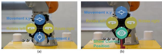
Figure 6: (a) Robot controls for the basic cues: yellow buttons rotate the gripper, top blue button moves the gripper on x,y axis and bottom blue button moves the gripper on the z axis. (b) Robot controls for the Advanced Cues: yellow buttons rotate the gripper, top blue button moves the gripper on the x,y axis, and the green button shows the current position of the gripper on the tabletop.
