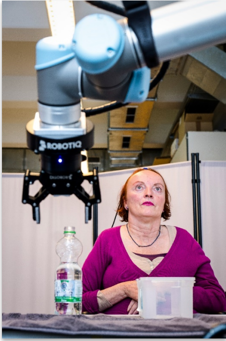
Figure 1: Tetraplegic user operating a Universal Robots UR5 robot arm with MARG head-mounted sensors [3].
