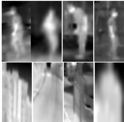
Figure 18. Misclassified samples. Upper row: False negatives due to low resolution, motion blur and pose variation Lower row: False positives in areas with a high vertical symmetry
