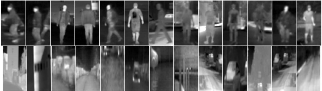
Figure 1. Example cropped images of the classification dataset. The upper row contains examples of pedestrians acquired under different temperatures and illumination conditions. The lower row contains randomly selected windows from images containing no pedestrians. For visualization purposes the contrast has been enhanced.
