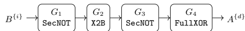
Fig. 5. An abstract diagram of B2X2A (Algorithm 4), t -NI gadgets are depicted with a single border.
