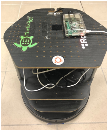
Fig. 6. The Turtlebot UGV with XBOX Kinect and Raspberry Pi computing modules.
