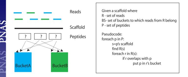
**Fig. S5.** Mapping peptides to geographic locations (sites). Schematic and pseudocode for mapping of peptides to a particular site are shown. The goal of this algorithm is, given this set of reads [color coded blue or green, depending on which bucket (site) they were recovered from], this set of peptides (boxes), and the coordinates from the scaffold (long black line), to determine to which buckets the peptides (boxes) belong.
