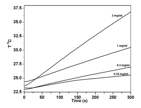
**Supplementary Fig. S3:** AMF induced magnetic nanoparticle hyperthermia in alginate microcapsules containing MNP. Four different concentrations of MNP; 0.25, 0.5, 1.0 and 2.0 mg/ml were encapsulated in alginate microcapsules and subjected to an AMF of 400 Oe. Efficient heating was observed in microcapsules containing 2 mg/ml of iron oxide.
