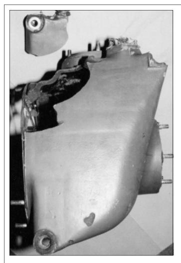
Failure of lower gearbox attachments was caused by excessive vibration and led to separation of the tail-rotor gearbox from the tailboom. (Photo: U.K. Air Accidents Investigation Branch)
