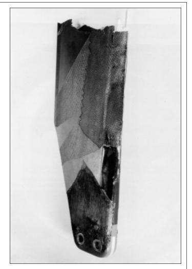
The damaged inboard (left) side of the white tail-rotor blade shows thermal delamination of the root area and general delamination outboard, including delamination of the leading edge from which the antierosion shield detached. (Photo: U.K. Air Accidents Investigation Branch)
