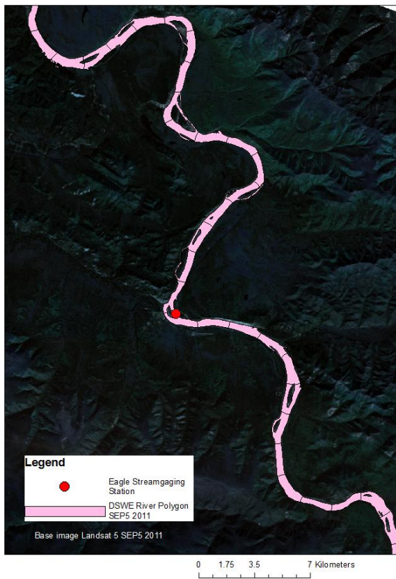
Figure 9 – Landsat image of the Yukon River at Eagle, Alaska, showing the Eagle streamgaging (red circle, latitude 64.79 deg. W, longitude 141.2 deg.) and the water surface extent in the river channel determined from DSWE in pink. The flow direction is towards the top of the image.
