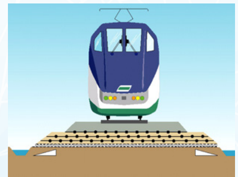
A railway line on soft soil with geosynthetics
